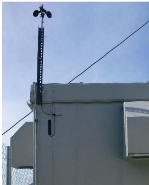
We have already installed wind meters to evaluate the wind potential for the future installation of additional small wind turbines.
